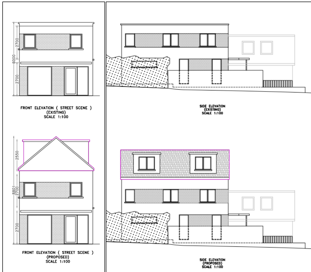
Figure 6.1: Existing and Proposed Elevations Demonstrating Roof Form
